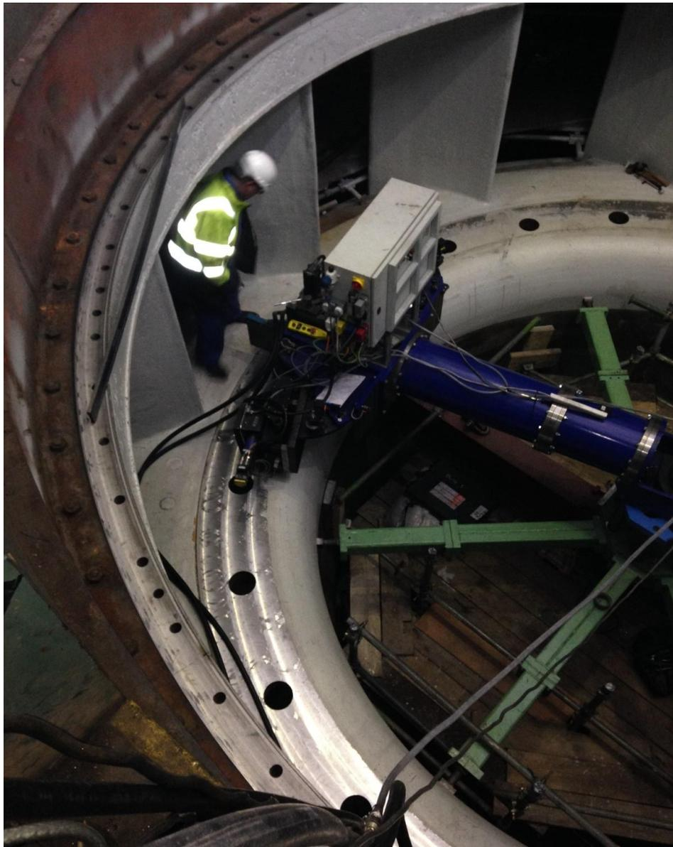
Laser Controlled Machining
